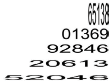
Figure 1. Character aspect ratios investigated in the legibility study. From top to bottom, aspect ratios (height/width) are 5.25, 1.26, 0.78, 0.46 and 0.26.
