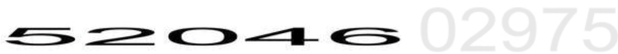
Figure 4. Left: Characters with a contrast of 0.9 and an aspect ratio of 0.26. Right: Characters with a contrast of 0.16 and an aspect ratio of 1.26. Both sets of characters would be expected to be equally legible.
